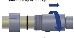
Slide the o-ring back towards the kink protection and ensure that it is flush against the o-ring seat oft he kink protection.
