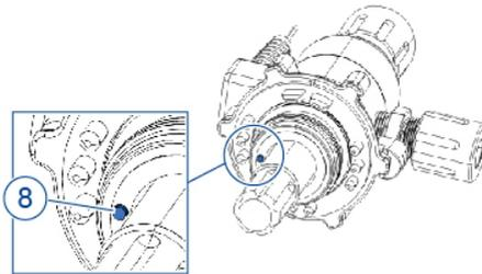
11. In the case of conductive dispense heads, check whether a conductive dip tube is installed and whether it is properly grounded. Follow the ATEX and OSHA instructions and regulations.
