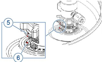
9. Align the code disk using the red or green orientation pins (5) and (6).
