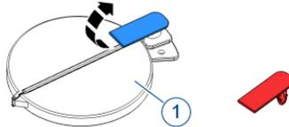
2. Open the tamper-proof cap and remove the red seal. Place both, if available, in the docking station on the system side (see Section 3.1).
