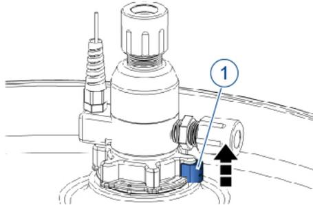
4. Slowly unscrew the dispense head via the tightening nut.
