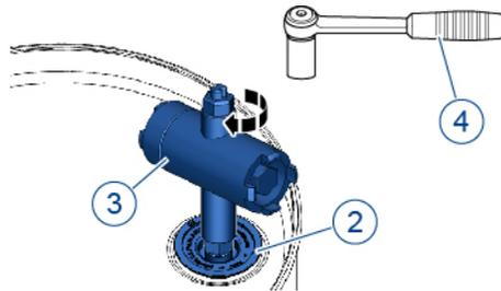
13. Take a torque wrench (4), place it on the bung wrench (3). Tighten the dip tube closure (2) to the correct torque.
