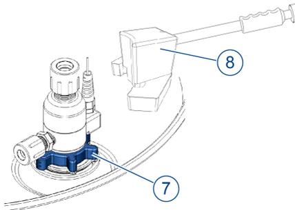
13. Check that the dispense head is completely and correctly mounted. This means that the dispense head must e.g. not be inserted at an angle.
