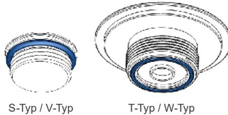
11. Place the dip tube closure on the dip tube opening.
